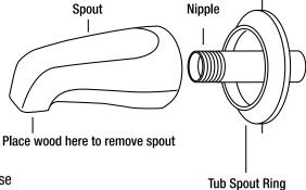
Reinstall spout by threading onto nipple by turning it in the clockwise direction. When installing the spout onto the nipple, hand tighten only. If alignment cannot be completed by handle, use the wood tool as in step 1. Ensure spout is centered onto the tub spout ring.
